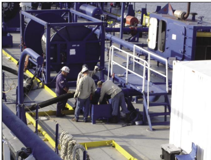
Response Personnel connect 8 in. hoses for oil transfer operations. Photo by MSRC.
